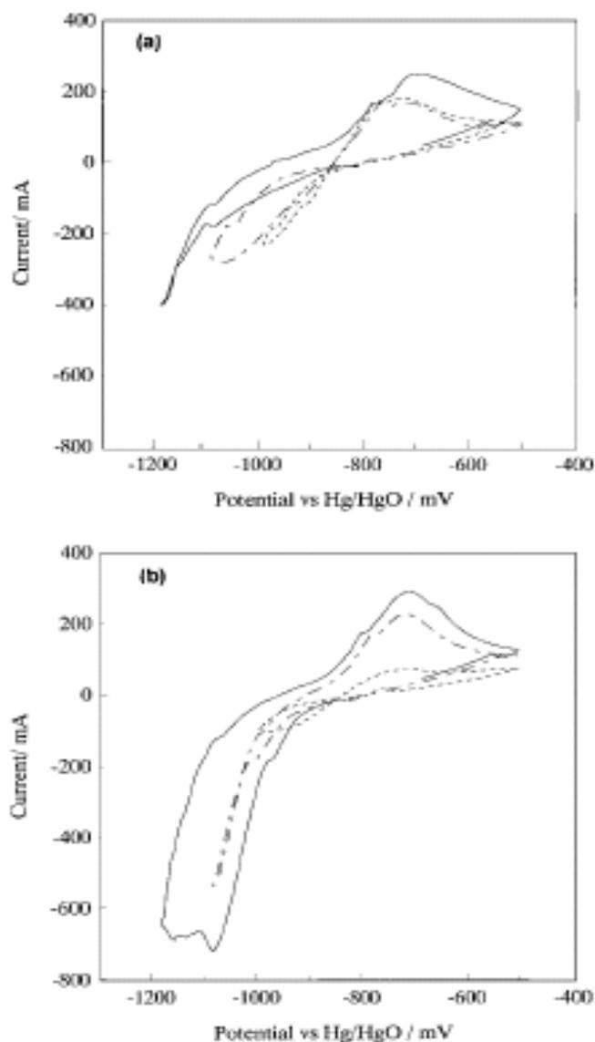
Fig. 3. Cyclic voltammograms of  $\text{Co}_x\text{B}_7\text{H}_2$  electrode sintered at  $200^\circ\text{C}$  with different cathodic switching potentials. Sweep rate  $5\text{mVs}^{-1}$ ; 20% KOH solution: (a) 1st cycle and (b) 5th cycle.
