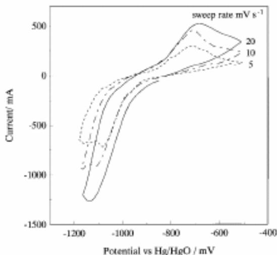
Fig. 5. Cyclic voltammograms of  $\text{Co}_2\text{B}_4\text{H}_2$  electrode sintered at  $200^\circ\text{C}$  with different potential sweep rates.
