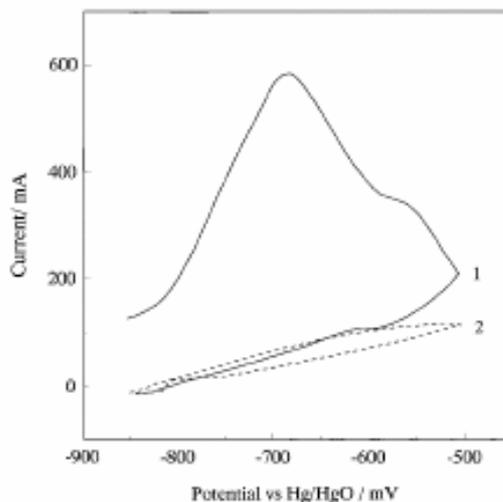
Fig. 4. Cyclic voltammograms of  $\text{Co}_2\text{B}_4\text{H}_2$  electrode sintered at  $200^\circ\text{C}$ ; the potential is swept only in the positive region towards the open circuit potential,  $E_{oc}$ . Sweep rate  $10\text{ mV s}^{-1}$ ; 20% KOH solution.
