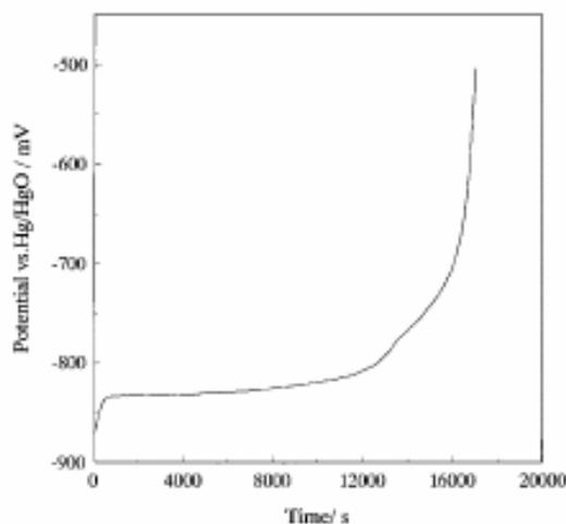
Fig. 6. Chronopotentiometric discharge curve for  $\text{Co}_x\text{B}_y\text{H}_z$  electrode sintered at  $300^\circ\text{C}$ . Discharge current density  $50 \text{ mA g}^{-1}$ .
