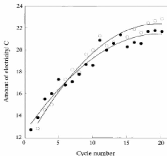
Fig. 2. Amount of electricity estimated by integrating the area under cathodic (○) and anodic (●) peaks in cyclic voltammograms obtained with  $\text{Co}_x\text{B}_y\text{H}_z$  electrode sintered at  $300^\circ\text{C}$ . Sweep rate  $5\text{mVs}^{-1}$ ; 20% KOH solution.
