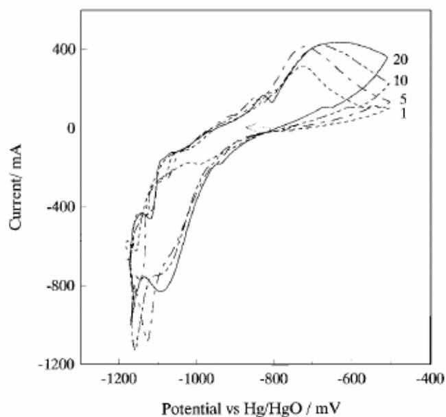
Fig. 1. Cyclic voltammograms of  $\text{Co}_x\text{B}_y\text{H}_z$  electrode sintered at  $300^\circ\text{C}$ . Sweep rate  $5\text{mVs}^{-1}$ ; 20% KOH solution. Figures inside note the cycle number.
